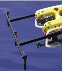
After installing the mounting frame(s) and sensors on the vehicle it is necessary to accurately measure (to an accuracy of 1mm) and record the positions and alignments of the various sensors, for entry into the system menu after computer switch on.
