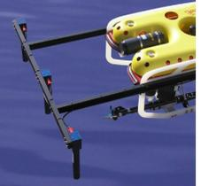
in the curved sections will contribute to the magnetic fields measured some distance away. If the cable has simple sinusoidal "S-bends" with wavelength much smaller than the distance between the cable and the sensors, this effect will result in the average position being calculated. However, if the "S-bend" wavelength is large compared to the distance between the cable and sensors, then the cable position calculated will be approximately that of the nearest point on the cable.
