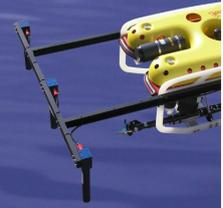
uniform wall magnetisation in a large pipe close to the sensor array (ex.24-inch pipe 50 cm below array) may result in such complex fields that the pipe mathematical model is inadequate and no solution may be found for pipe position. Pipe/cable size has no effect in the ACTIVE D.C. or ACTIVE A.C. CURRENT modes.
